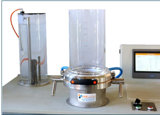
Sheet former column & white water tank
